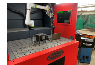
On-torch fume extraction for cobot workstation with FE GoMax
